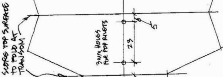
ANK! FOOTY DESIGN PATTERNS FOR HULL ASSEMBLY JIG PART 1 OF 2
