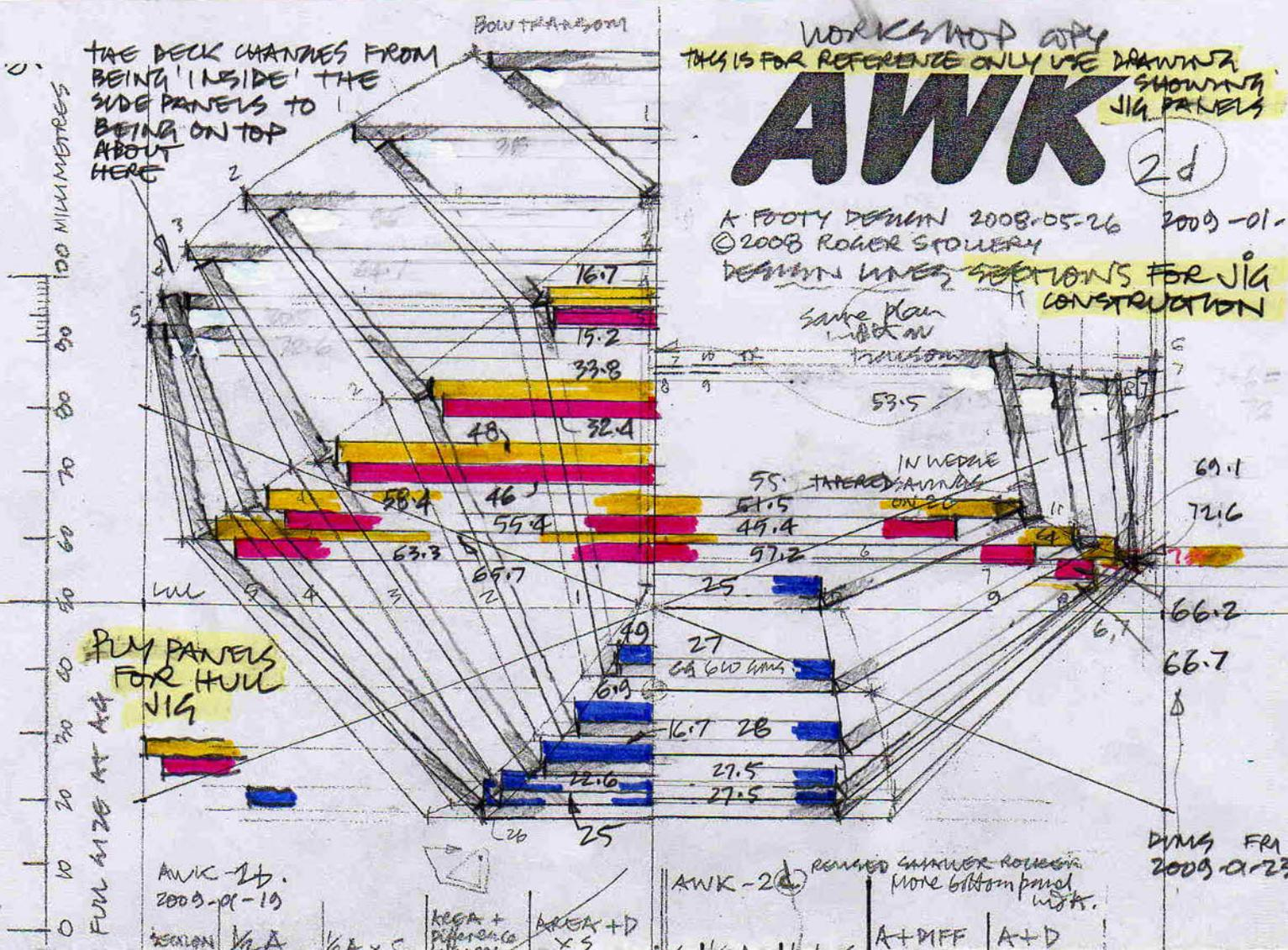
Please note that this is for reference and to explain the construction of the hull jig. The hull jig panel patterns shown on the other drawing are 'as built' and should be followed in preference to any dimension on these sections.
