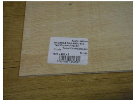
IMAGE 2) Starting Plywood board 1200x400x5 mm
