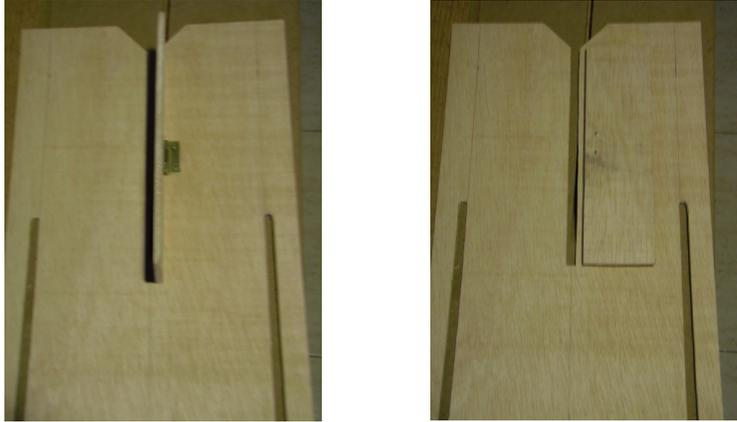
IMAGE 7) Rudder board open and closed
